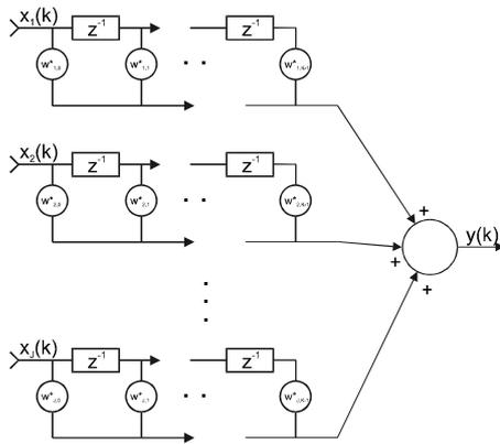
Figure 6. Beam forming signal flow chart for broad band signals.
