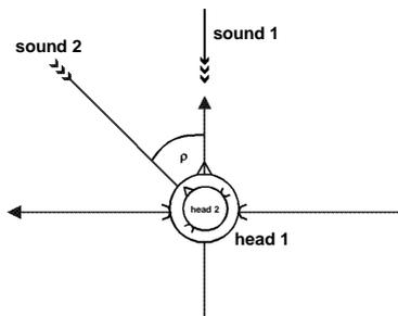
Figure 1. The subject's head movement results in different HRTF filters for a static sound field (sound 1, sound 2). This figure demonstrates that two static sound sources demand different filtering for head position one and two after rotation.
