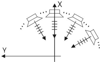
Figure 3. Reproduction with a symmetric loudspeaker layout.
