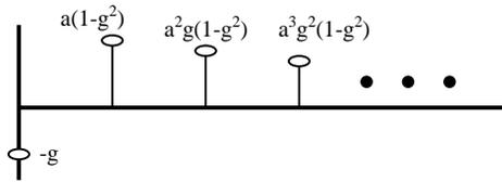
Figure 8. Impulse Response of Absorbent All-Pass Filter
