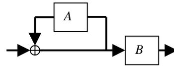
Figure 7. Energy Gain Representation of Late Reverberation Network
