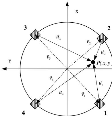
Figure 1. Four loudspeakers system configuration.
