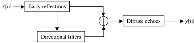
Figure 5. Reverberation block diagram.
