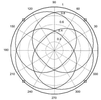
Figure 3. Polar diagram of loudspeaker gains,  $r=0.3$ .
