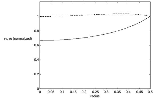
Figure 4. Evolution of the amplitude of normalized velocity vector (solid) and normalized energy vector (dotted) with the radius.
