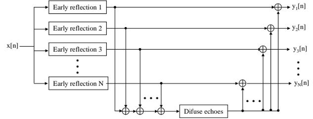
Figure 8. Directional reverberator block diagram
