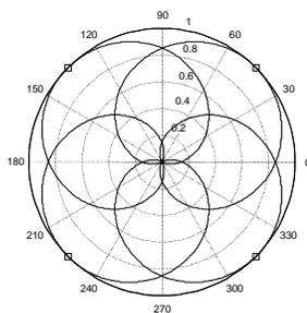
Figure 2. Polar diagram of loudspeaker gains,  $r=0.5$ .
